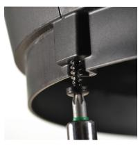
Remove one of the screws using a T-15 Torx bit.
