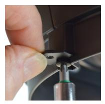
Attach the mounting tab to the front ring. Tighten the tab so that it is snug but still can be moved to align with the accessory's mounting holes.
