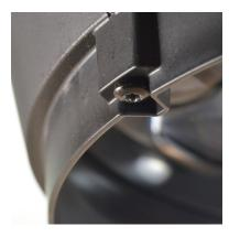
Locate the three screws which attach the fixture's plastic front ring
