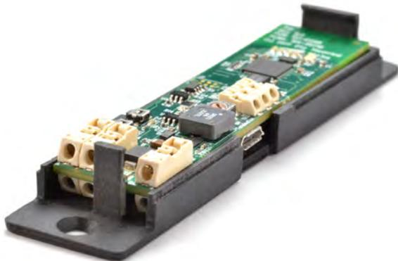
**QolorFLEX® 2x2.5A Multiverse® Dimmers are small, constant voltage, two-output dimmers designed to be mounted in small spaces such as props, costumes, wands, and candles.**
