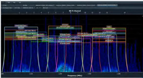
A sample real-life crowded radio spectrum, shown in RadioScan software program.
