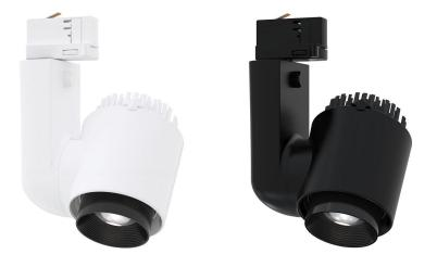
The Jade Zoom is a versatile and powerful LED lighting fixture. With a zoom range from 9° to 58° (Bridgelux) or 11° to 67° (Xicato), it is ideal for museum, gallery, or high-end retail lighting. The advanced optical system ensures uniform light quality, while the choice of LED light sources allows for a perfect fit to the lighting plan.
