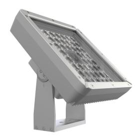
The Quartz is an IP67 outdoor lighting fixture which can be configured in many configurations. It is made from CNC cut, massive aluminium. The ventilation gland with Gore-Tex membrane minimizes the risk of condensation. Up to 8500 Lumen effective light output from a compact, 25 x 25 cm fixture.
