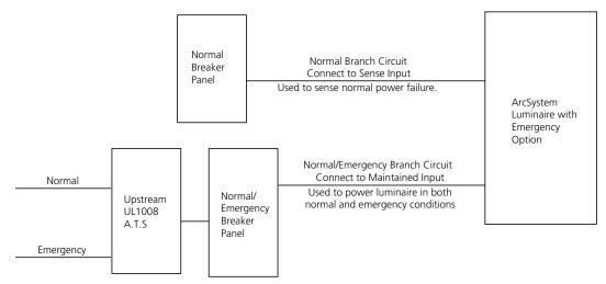
The sense input is used to detect whether normal utility power has been lost. This will force the luminaire on at 100% intensity running from the maintained supply. There is no control of the luminaire via wired-DMX until normal utility power is restored to the sense input.
