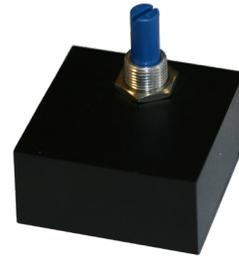
The DM1 dimming module allows basic intensity control of up to 40 BlueBeam or BlueDome LV fixtures. The module is designed to be installed into an electrical faceplate or panel of your choosing and features the same three terminal connections as the fixtures (power, ground, control) for ease of commissioning. See BluesSystem installation guide for further information on wiring configuration options.
