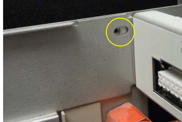
Slide arm clips in place to ensure proper screw alignment
