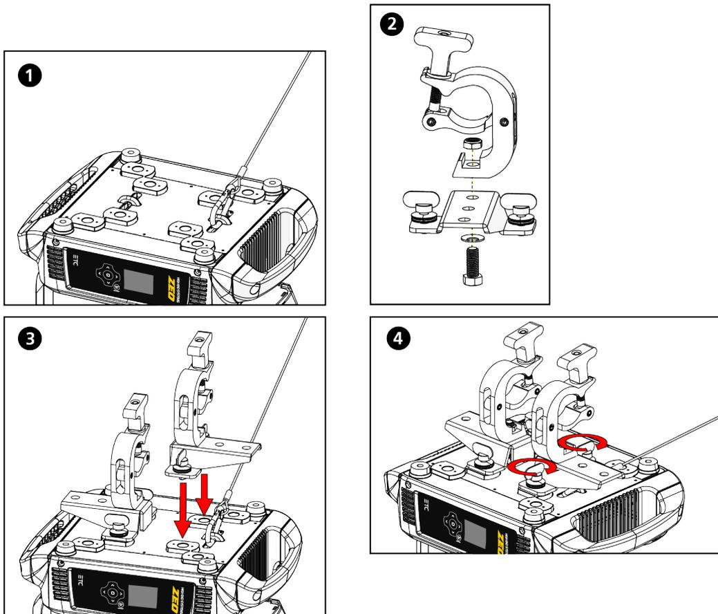
1. Attach the provided safety cable through one of the two attachment points on the bottom of the fixture upper enclosure.
