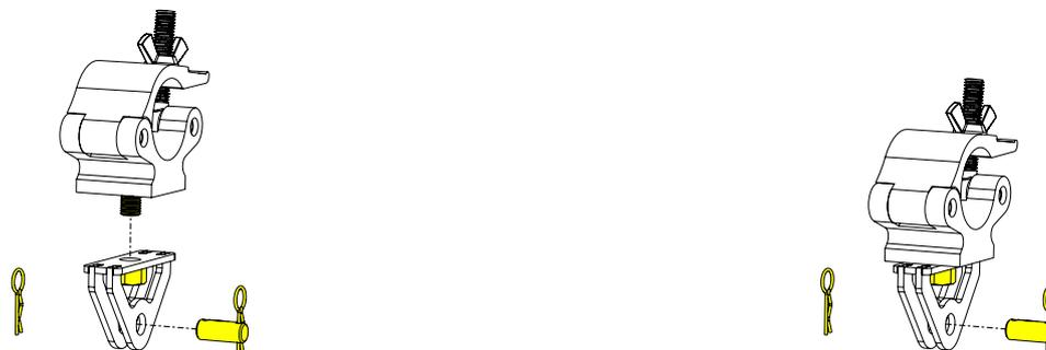
Secure the adaptor to the SBAR40 and replace the pin.
