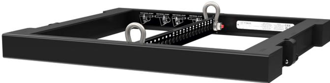
The T12GRID is used to vertically array TORUS for up to 6 cabinets. Cabinets may be flown from the T12GRID inverted allowing stereo arrays to be mirrored with the high frequency horn either to the left or the right.
