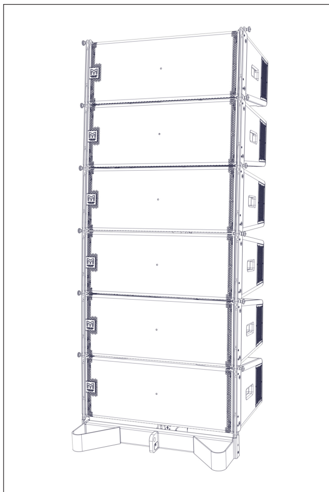
Fig. 52 - complete ground stack
