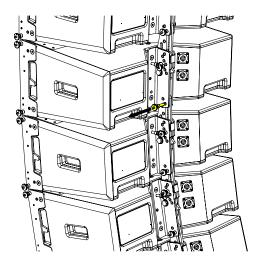
Remove the front locking pins from the fifth cabinet at each side. Ensure the cart is fully grounded when removing pins.
