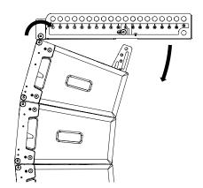
Insert the pin into the LINK hole on the flying frame.
