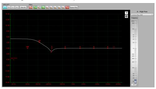
The output EQ is greyed out as it is used to apply the EQ created by your DISPLAY project, however the high-pass filter is available for adjustment so you can determine the crossover point between the WPS array and your subwoofers.
