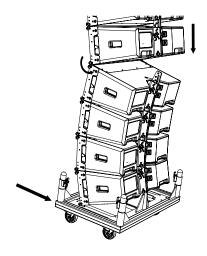
Insert a pin in the rear rigging bracket at the correct angle. Allow the bottom four cabinets to swing back down and insert rigging pins into the LINK and LOCK positions on the fourth cabinet. Connect the cable loom and any link cables as required to the lower four cabinets.
