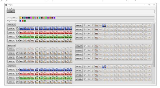
Once the system is configured to your satisfaction the 'Master Overview' gives a complete picture of even the most complex system allowing you to monitor all metering and access commonly needed functions such as gain and mute.
