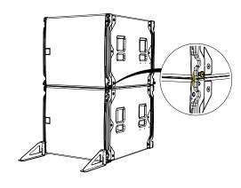
Replace the pins locking the link into the WPSGRIDt.
