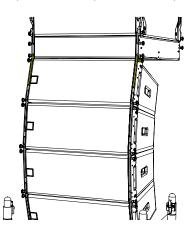
Insert the pin into the LINK hole on the flying frame.
