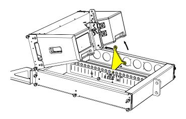
Repeat the process for the second cabinet, removing the link pins and lower it onto cabinet 1.
