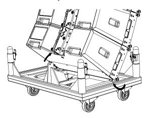
Remove the LOCK pins from the rear rigging bracket on the bottom four cabinets.
