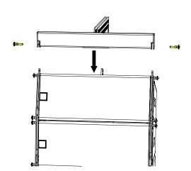
Insert the link pin at the front rigging position on each side.
