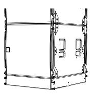
Position loaded WPS transport cart underneath the array, remove the top and poles and prepare the cabinets to be added to the array.
