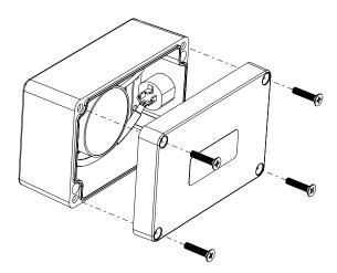
Using the PZ2 Pozidrive screwdriver, unscrew all four lid screws until the lid can be removed from the base of the box. Note that the screws do not have to be completely removed from the lid, they can remain captive in the lid to prevent them getting lost.
