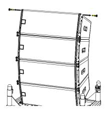
Raise the front links on the fifth cabinet and insert the link pins on both sides in the fourth cabinet.
