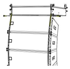
Lift the array to allow the WPS cabinets to be suspended on the front links. The array will pivot on the front and can now be attached to the spine of frame using the rear WPS link.
