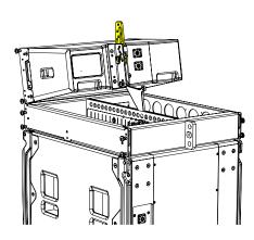
Secure the front of the second cabinet with link pins on both sides.
