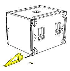
If needed place a second SXCF118 on top and remove the pins from the stow position, rotate the links and align them with pin holes on the top cabinet.
