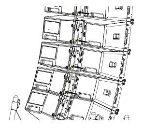
Raise the front of the cart and pin it in position to the front of the array.
