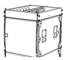
Remove the link pins and lower the WPS cabinet onto the frame until the two up-right bars on the frame locate in the front rigging assembly of the WPS. Insert the link pins in the WPS rigging assembly to secure the front rigging system.
