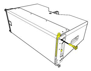
Inter-cabinet angles are set using the rear rigging assembly. This consists of a link bar with indexed holes which can be moved upwards and secured with a link pin in one of eight available positions:  $0.5^{\circ}$ ,  $1^{\circ}$ ,  $2^{\circ}$ ,  $4^{\circ}$ ,  $6.5^{\circ}$  and  $10^{\circ}$ .
