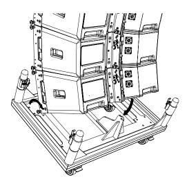
Repeat at the front of the array supporting the cart and removing the pins holding the cart to the array.
