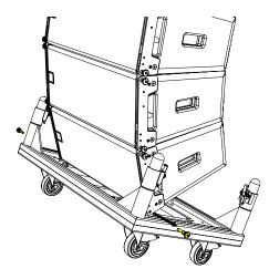
Raise the array to the final trim height. The use of either one or two motors and rigging positions (WPSGRIDt only) allows both negative (down-tilt) or positive (up-tilt) array angles to be easily achieved.
