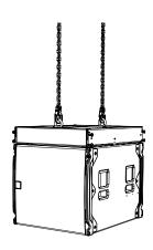
Replace the pins to link and lock the SXCF118 securely to the WPSGRIDt.
