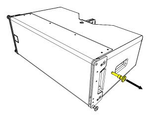
It is important to check that the central button does not remain depressed once you have put it in place as this would indicate that the pin has not been pushed all the way into position and the ball bearings at the end of the pin have not been able to pop out and rigging the pin in place. If the pin is not locked the array is unsafe. The pin MUST be repositioned until it is securely locked in place.
