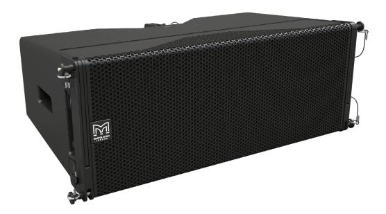
WPS is a new breed of small-format optimised line array which brings innovative acoustic design, ultra-high performance and coverage consistency to a wider range of users, applications and budgets than previously possible. The three-way, passive system features reflex loaded low-frequency, and horn-loaded mid and HF sections to raise efficiency and increase output. Its high efficiency acoustic design can equal or outperform larger, direct radiating designs
