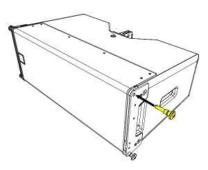
Pull the pin clear using the wide flange whilst your thumb depresses the central button.
