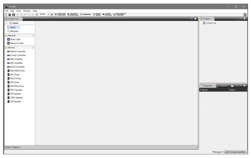
The application opens with a blank system diagram. It is possible to add products manually using the 'Palette' on the left, but this has limited use. However, in practical applications the 'Discover Devices' button is used.
