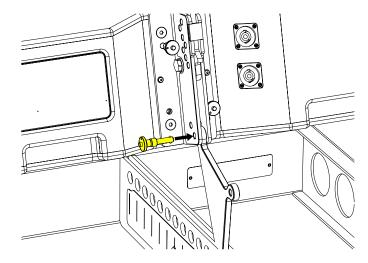
Secure the front of the second cabinet with link pins on both sides.
