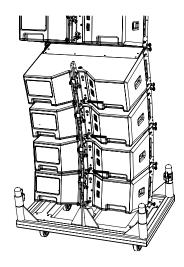
Raise the array clear of the transport cart, allowing access to the rear of the array.
