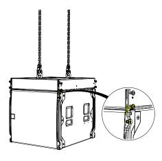
Remove the pins from the stow position, rotate the links to line up with the pin hole position on the SXCF118 above.
