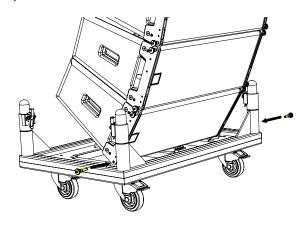
Pin the cart to the rear rigging bracket of the array.
