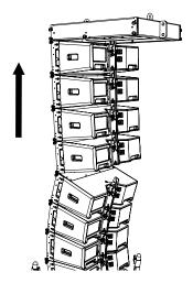
Swing the bottom four cabinets (which will now be a rigid array due to the rigging pins) backwards until butted against the upper half of the array.
