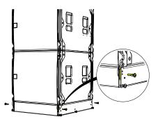
Replace stow pins to look the links into position. Use the spare pins on the WPSGRIDt to lock the links to the SXCF118.
