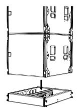
Remove the pins from the stow position, rotate the links to line up and align with the pin hole position on the SXCF118 above.
