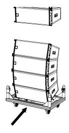
Lower the array and align the front rigging assemblies of the fourth cabinet with the front rigging points of the fifth cabinet.
