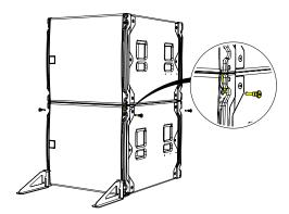
Remove the pins, rotate the links to line up and align with the pin hole position on the WPSGRIDt.
