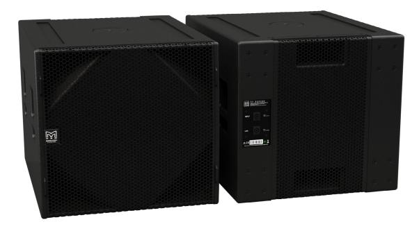
Designed for touring sound and installations, the SXC118 and it's flown variant, the SXCF118, is a compact, high performance cardioid subwoofer. It features an 18" (460mm) forward facing driver and a 14" (356mm) rear facing driver, each driven independently by separate amplifier channels and DSP. Each driver has its own chamber with optimised bass reflex porting.
