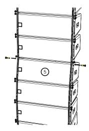
The cabinet angles will open as far as the pins will allow to the angle that has been pre-selected. Insert rigging pins at the LOCK position on the remaining cabinets.
