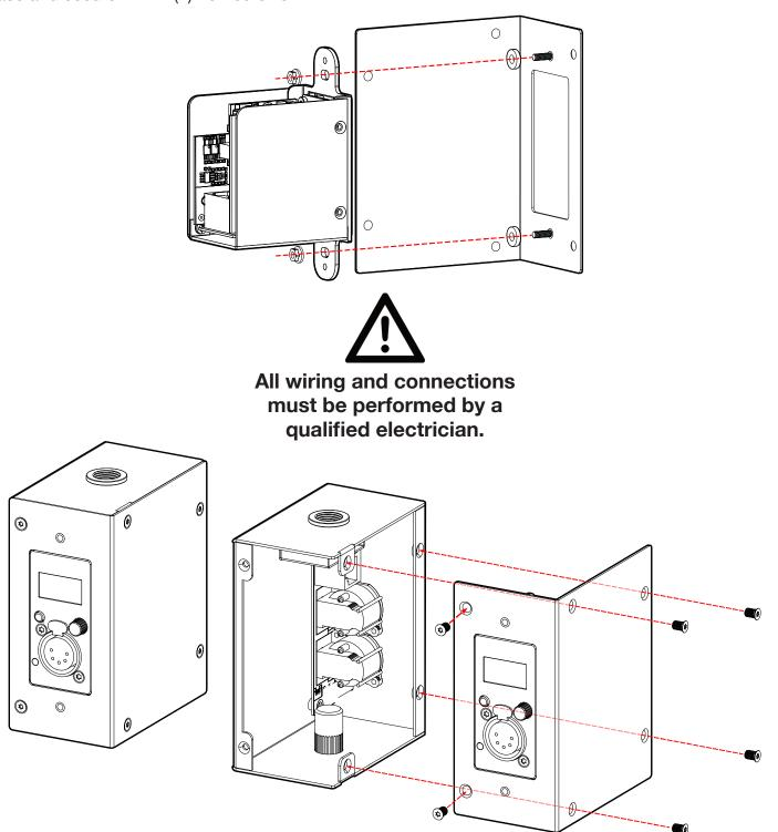
Once a qualified technician/electrician has reconnected the control surface panel with the power and data connectors, the control surface panel can then be mounted and secured to the base assembly with (6) torx-screws.
