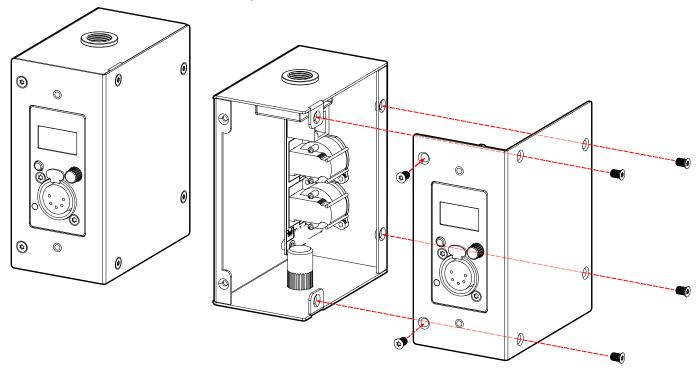
1. Remove (6x) torx-screws securing the control surface panel to the integrated multi-use mounting-bracket and separate. A qualified technician/electrician can then disconnect the data and power connectors from the control surface panel to the mounting case.
