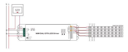
Note: all 4 channels are controlled together under this mode.
