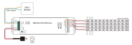
Note: The control gear will be discovered by DALI master as a DT6 device, 4 channels controlled together.
