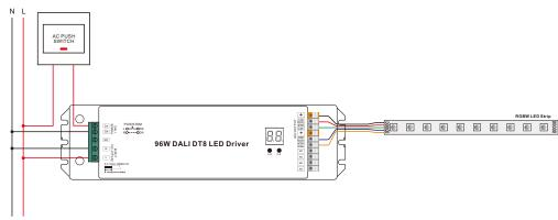
Note: brightness of both RGB & W LEDs can be controlled, color control only applicable to RGB LED under this mode.
