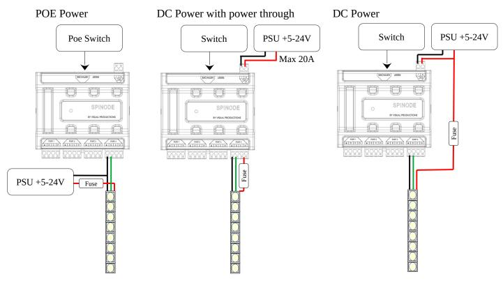
The power through feature allows you to power your led strip from the SpiNode DC power supply.
